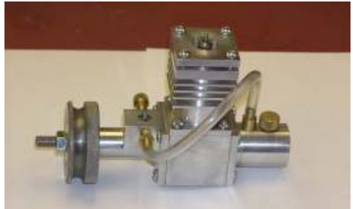
First year Pine Technical College manufacturing student Nick Farrand displayed the functional model engine he completed for class requirements using his CAD drawings.
